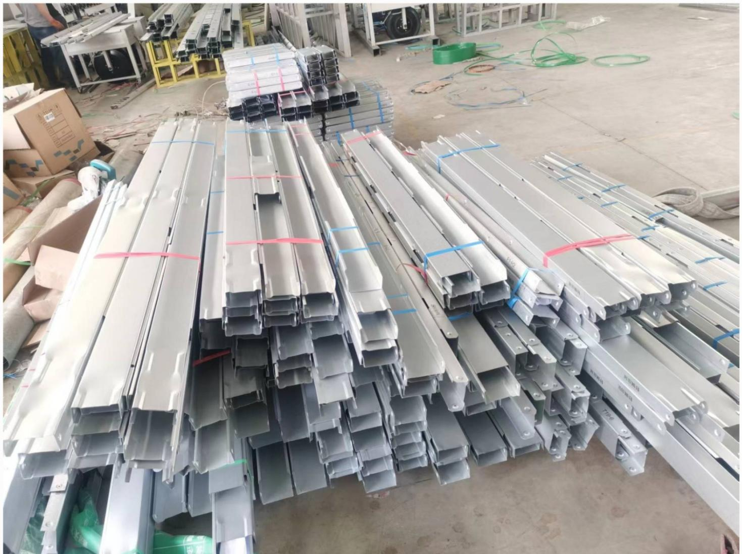
Material Selection: High-zinc steel with a zinc coating  $\geq 275\text{g/m}^2$ , formed through hot-dip galvanizing to create a dense oxide layer, providing over 50 years of corrosion resistance in humid environments.
